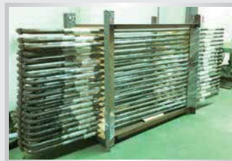
CDQ設備爐管 (Boiler Tube)
