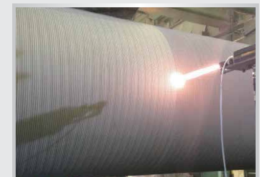
複捲軸施工 (Spraying on Winder Roll)
