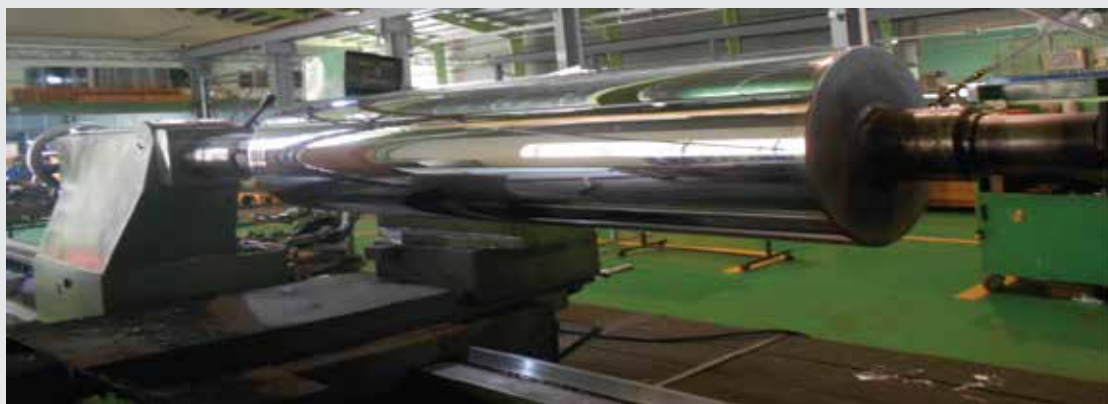
鏡面輥機台上加工 Machining mirror surface roll
